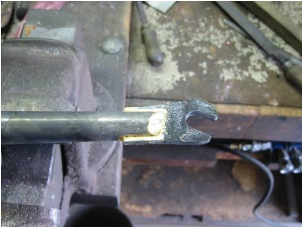
Flux washed off the front tip after brass brazing
