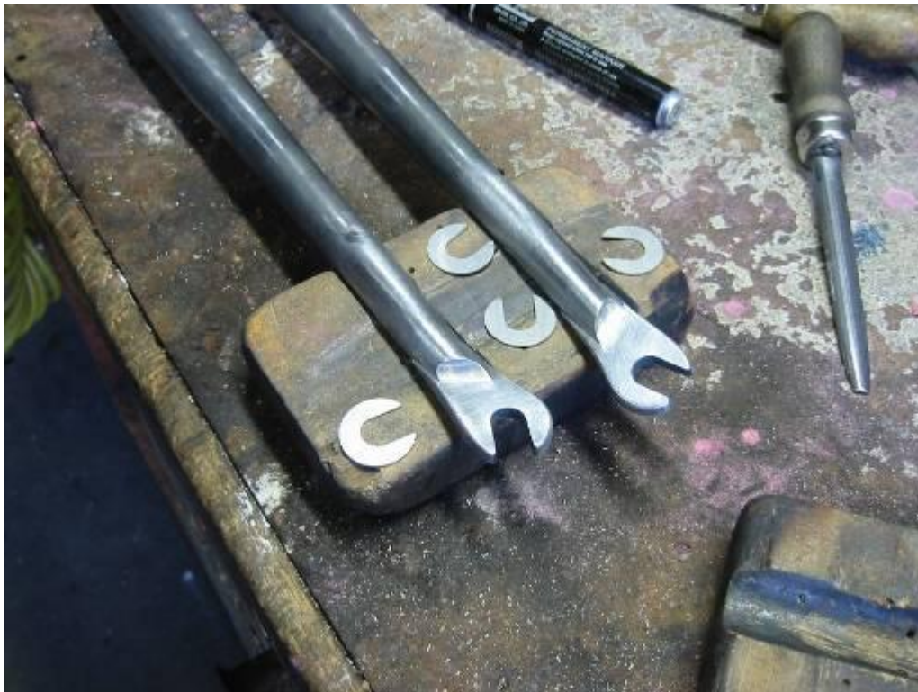
Front fork blades ready for the stainless steel wheel bite facets to be silver brazed to the tips.
