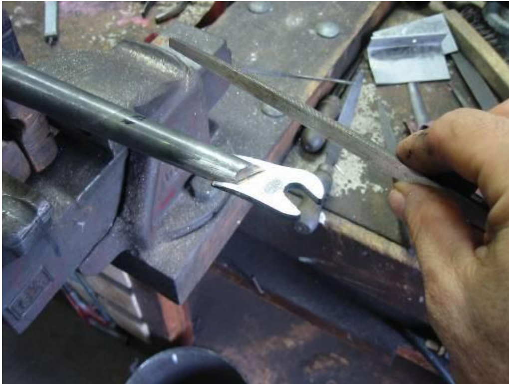
Filing and shaping. Better to have lots of material to remove than not enough to get the sweet shape
