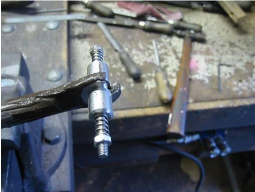
The special Llewellyn facet brazing thingie, made from titanium {so the silver does not stick}
