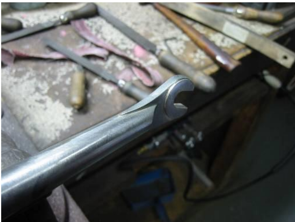
A bit more filing and the result is sexy smooth points along the fork blade.
