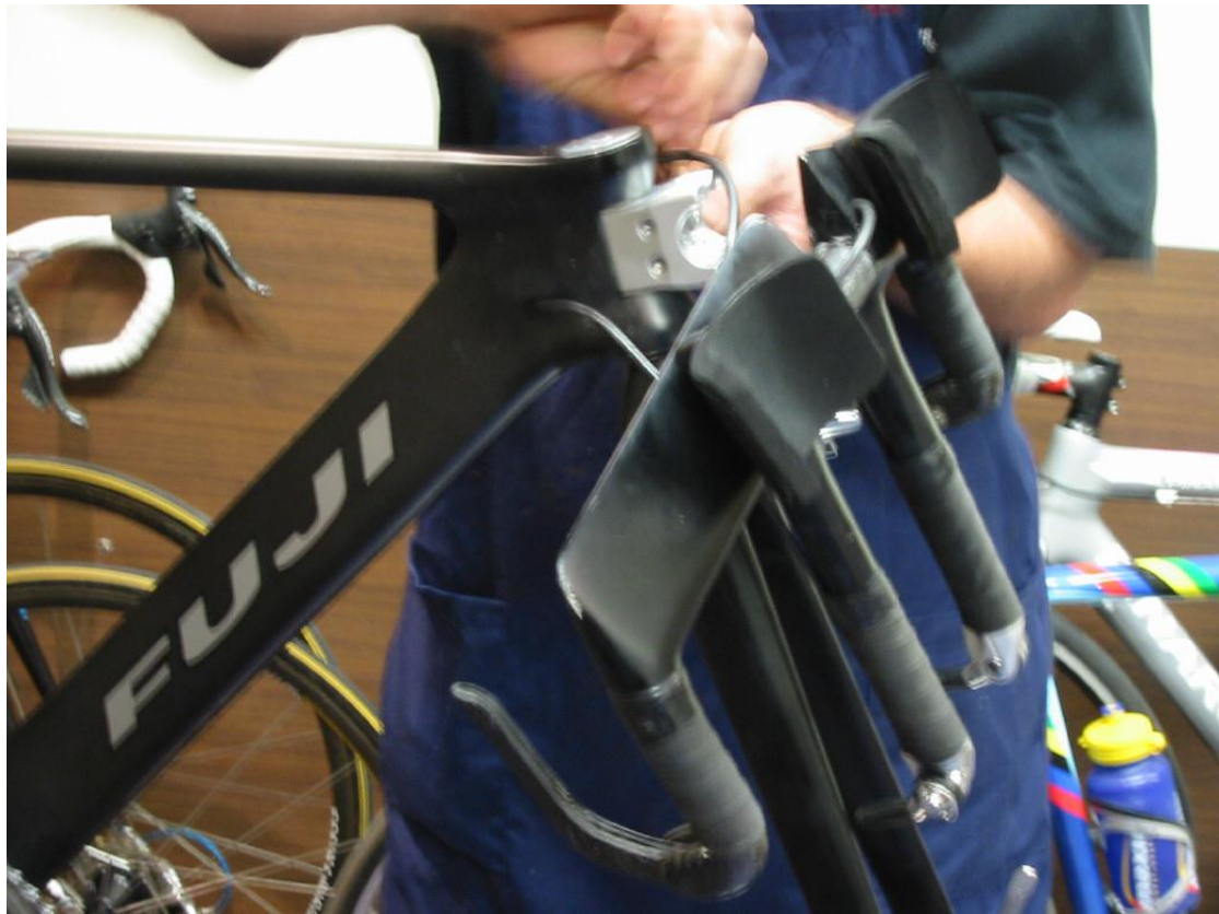
Fitting the new properly made stem and it went in smoothly. This was very pleasing. {Fuji team decals, privately made Swiss bike.}
