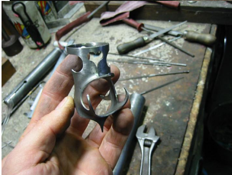
The lugs have been cut from "Pacenti Artisan lugs", the polishing of these stainless lugs occurs after brazing. Four days work for the three lugs
